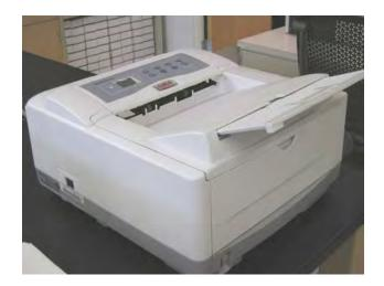
Other compatible printers may be used. Intox has reported that not all printers are compatible, they must be PCL5 or lower. Some network printers are an option with the upgraded EC/IR's.
