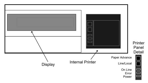
Note: These lights are associated only with the Internal Printer and have nothing to do with the Instrument
